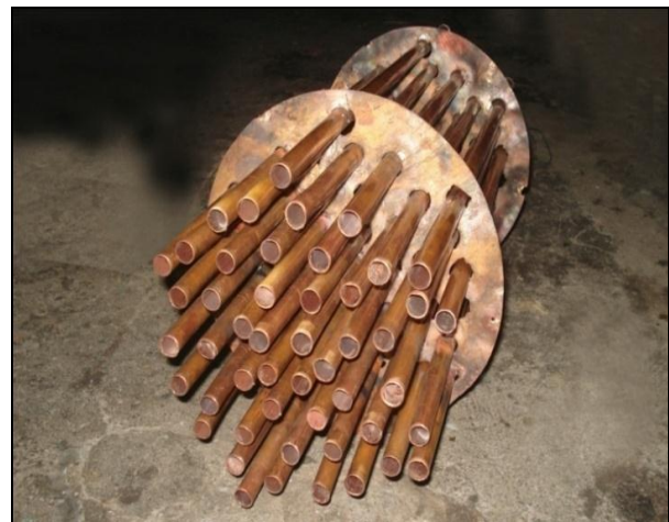
Fig 2: Fabricated PCM Storage Tank [3]
