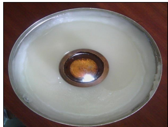
Fig 7: Steel Container with Water and Paraffin Wax
