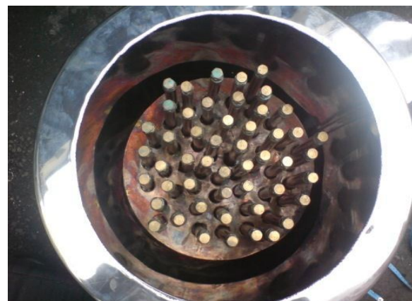
Fig 2: Fabricated PCM Storage Tank [3]
